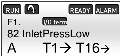
Figure 7.1-4, Low pressure alarm on the NXP panel
