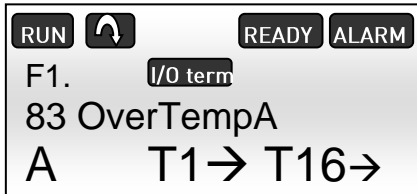
Figure 7.1-2, High temperature alarm on the NXP panel
